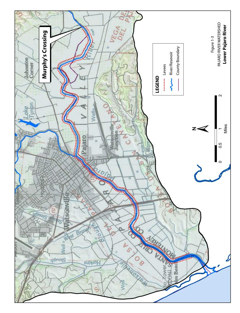
raised to provide additional protection. New levees filled in gaps and extended the coverage area. The current levee system provides protection against approximately a 25-year storm.
