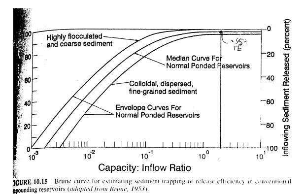
Figure 1. Brune Curve estimation of Hernandez Reservoir Trap Efficiency.
