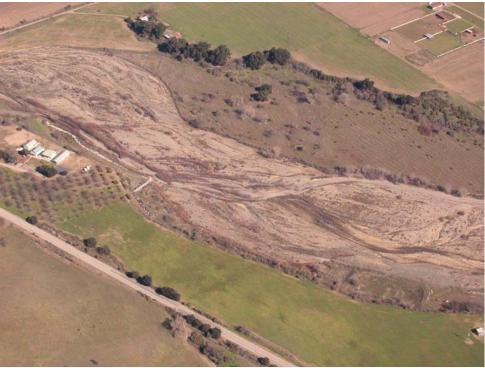
Figure 3. San Benito River, showing braiding, mobile riverbed and bank erosion.
