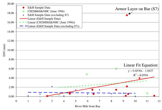
Figure 32. Comparison of E&H and CH2MHill (CH2M HILL 1997) median grain sizes for the lower Pajaro River.
