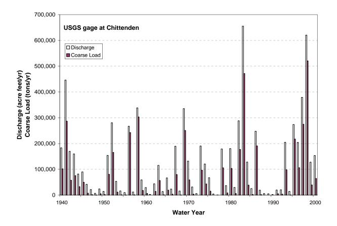
Figure 5: Discharge of water and coarse sediment load at Chittenden, by water year.
