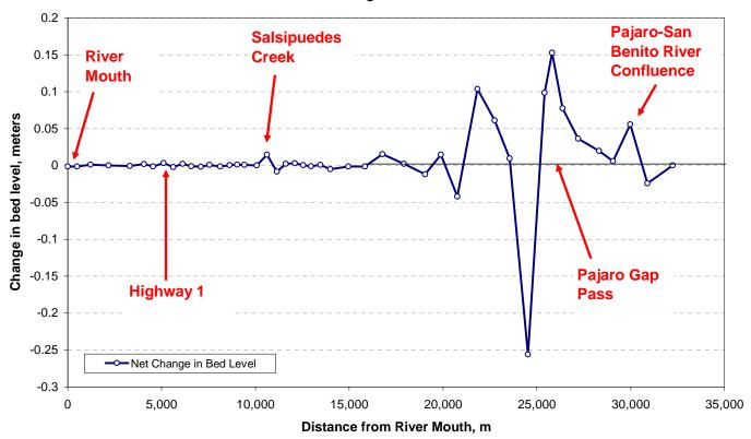
Figure 3: Results of Simulation #3. Difference in the end-of-flood bed profile along Pajaro River for a 50% increase in channel hydraulic roughness, as compared to the end-of-flood bed level for the Existing Condition model.
