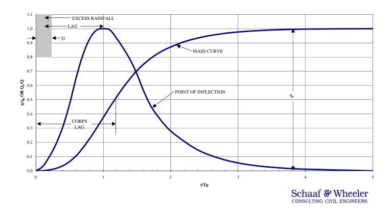
The SCS definition of lag is shown graphically in Figure 7.2. It is different than the one the Corps uses. For use in the PRO-FLO model, the Corps of Engineers lag is converted to the SCS lag by multiplying the results of the above equation by 0.8625 and subtracting half of the one-hour unit time of the unit hydrograph.
