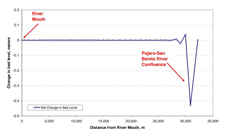
Figure 5: Results of Simulation #5. Difference in the end-of-flood bed profile along Pajaro River for a 20% decrease in total sediment load, as compared to end-of-flood bed level for the Existing Condition model.
