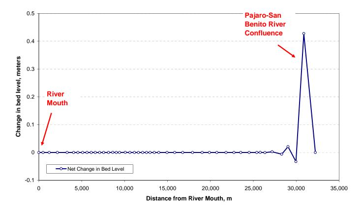
Figure 4: Results of Simulation #4. Difference in the end-of-flood bed profile along Pajaro River for a 20% increase in total sediment load, as compared to end-of-flood bed level for the Existing Condition model.
