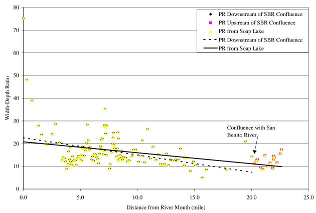
Figure 29. Width/Depth Ratio for Pajaro River from Downstream of Soap Lake to Outlet.
