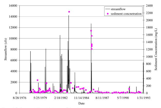
Figure 1. Sediment and Water Discharge at Chittenden gauge.
