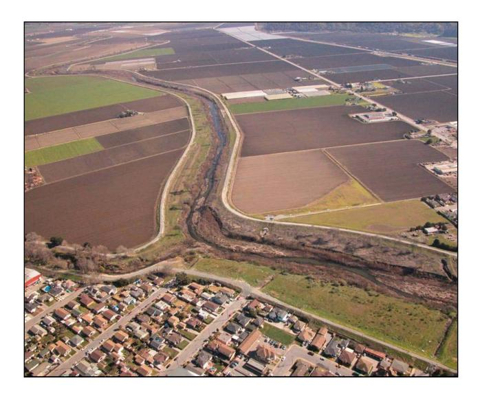
Figure 3: Aerial photograph of confluence of Pajaro River and Salsipuedes Creek illustrating the levees, main channel with sand bars, and the very small floodplain between the top of the channel bank and the levees. View looking upstream. A residential area of Watsonville is in the bottom of the photo.
