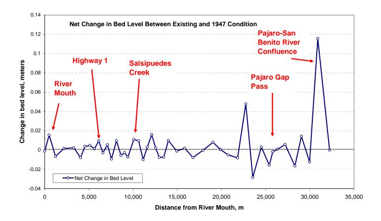
Figure 2: Results of Simulation #2. Difference in the end-of-flood bed profile along Pajaro River for the 1947 discharge hydrograph, as compared to the end-of-flood bed level for the Existing Condition model.
