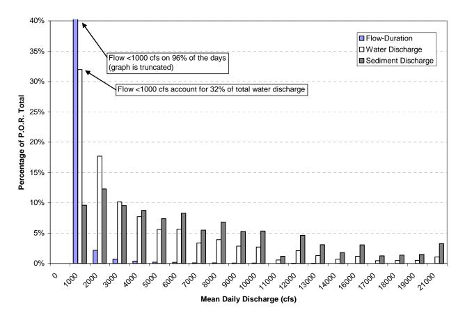
Figure 6: Histogram showing the percentage of total sediment and water discharged by discharge class (1000 cfs per class interval).
